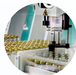
MPS Dual Head WorkStation with SPE and centrifuge for automated clean-up of QuEChERS extracts
