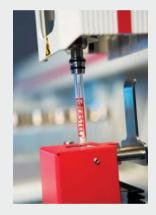
you can pack the tubes yourself with the adsorbent(s) of your choice. Since the trap is back-flushed during desorption, multi-bed adsorbent tubes can be used in order to cover a wide range of analyte boiling points and polarities in one analysis for improved flexibility and productivity.
