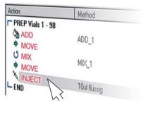
MAESTRO Software enables Sample Prep by Mouse-Click. All sample preparation steps are conveniently and easily selected from a drop down menu and added to the method. Example:
